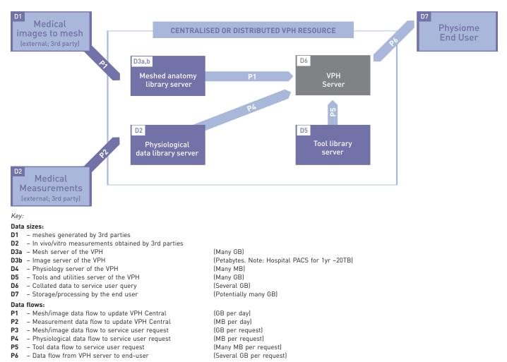
Figure 6.3. Notional data storage and data flows to service a simple VPH request.
